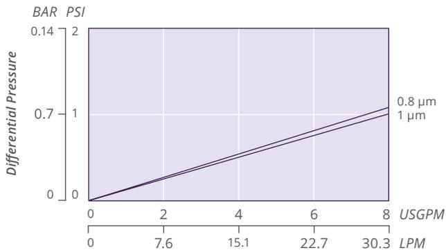
*For liquids other than water, multiply pressure drop by the fluid viscosity in centipoise*
